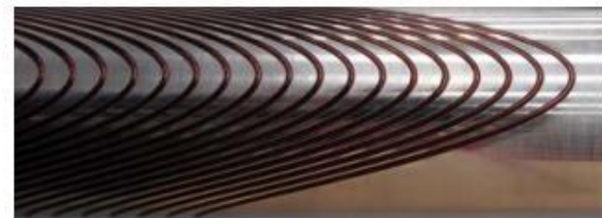
fig. 1. Top: winding of a double helical coil for generating a quadrupole magnetic field. Bottom: a winding test with a dummy wire.
