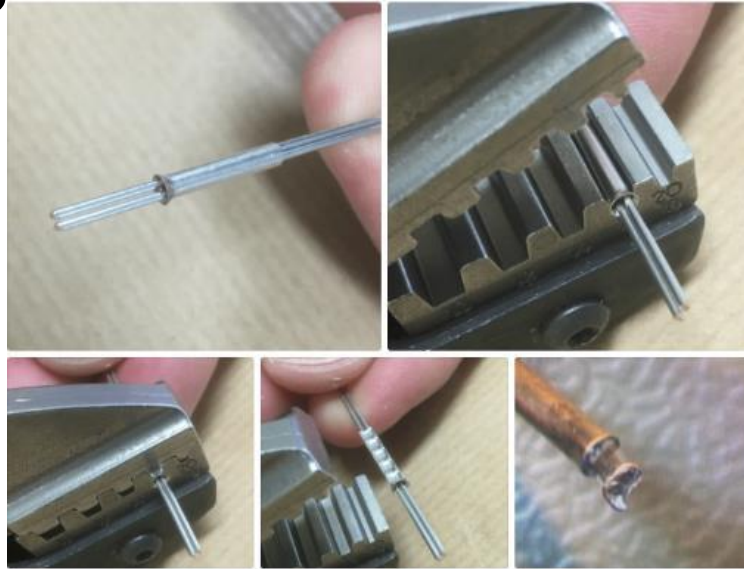
600A joint Copper tube tined with solder, crimped, and soldered,
