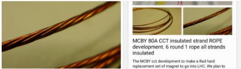
MCBY rope conductor using 7-0.3 mm strand
