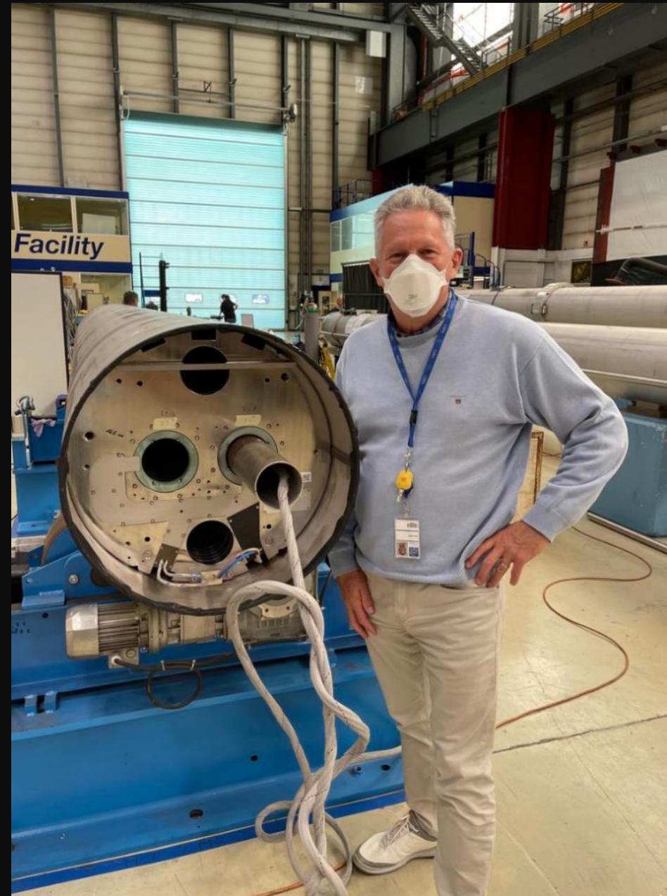
1st CCT to go into LHC MCBRD CCT at CERN
