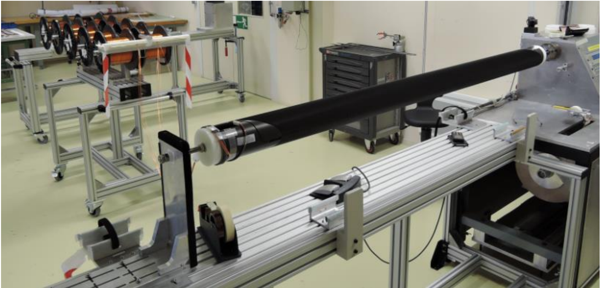
10 spools with insulated wire, Wire cleaning, Hard anodized aluminium 6082-T6 CCT former
