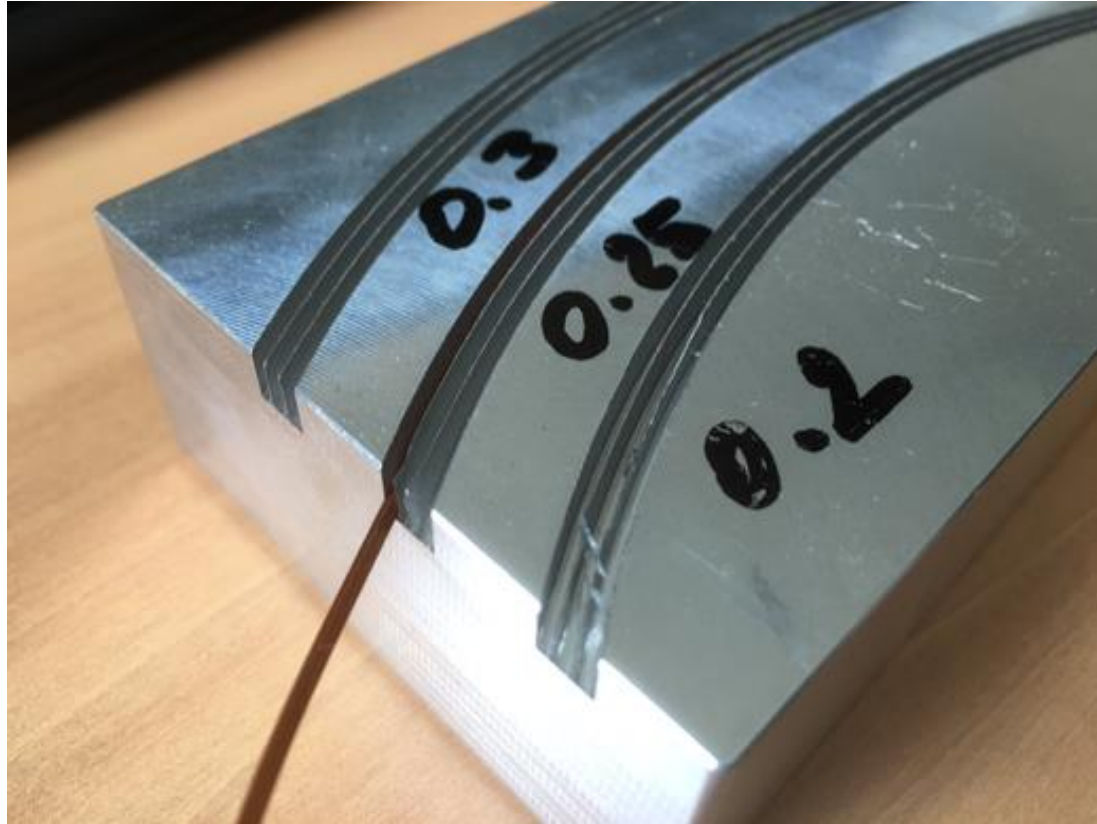
Min wall 0.3mm with 2mm wide channel
