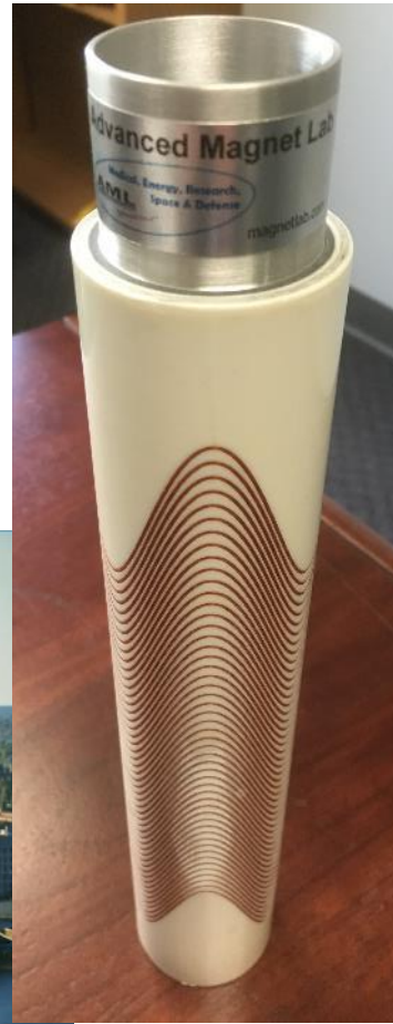
Figure 5: A few turns of epoxy impregnated coil, with a Lexan cover, show typical turn geometry. Insulation is provided by the web of the coil support grooves and the epoxy impregnation.
