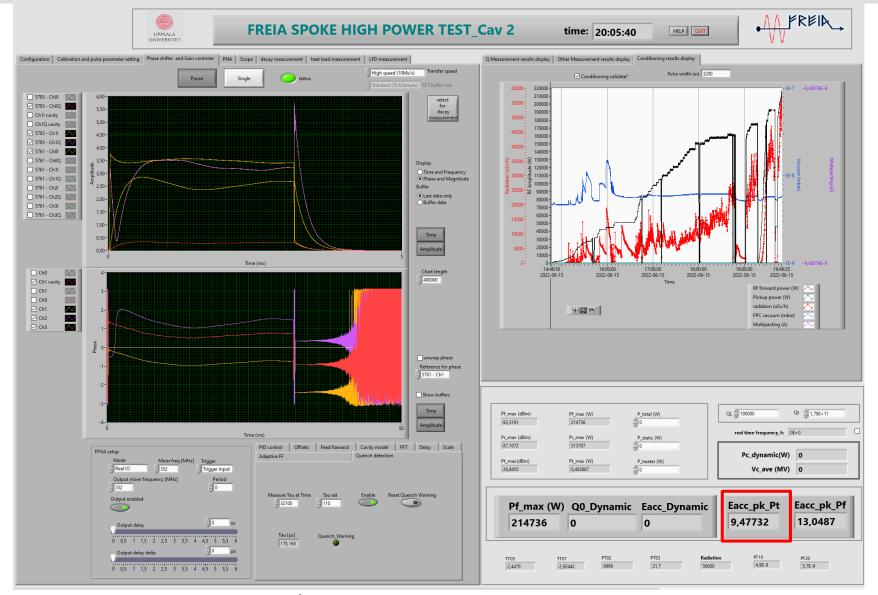
We stopped at 9.5 MV/m due to very high heat load with X-rays9
