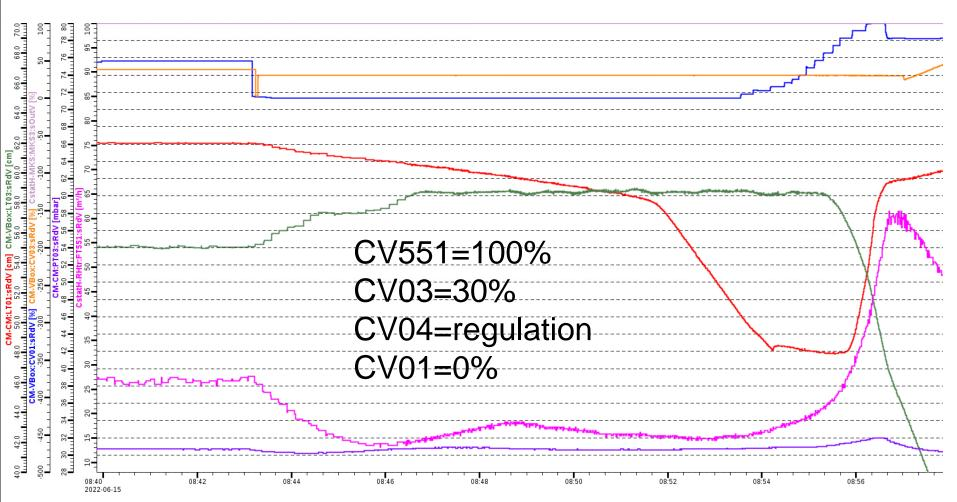
GHe exhaust flow FT551 = 16.03 m3/h (std dev 1.17 m3/h) → **17.15** +/- 1.25 W
