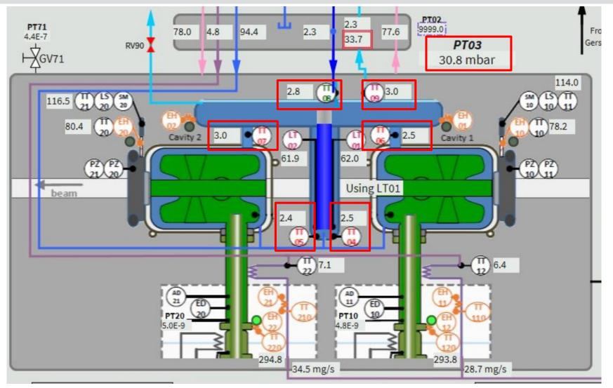
30 mbar is confirmed by other pressure gauges but all the CERNOX in CM11 show warmer value corresponding to around 100 mbar
