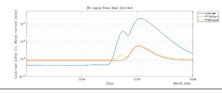
We performed final leak test of the insulation vacuum due to ESS' findings in CM08  $\rightarrow$
