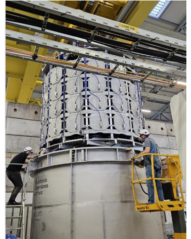
Support cage with mPMTs being inserted last week in the outer water container in the East Hall t9 beam
