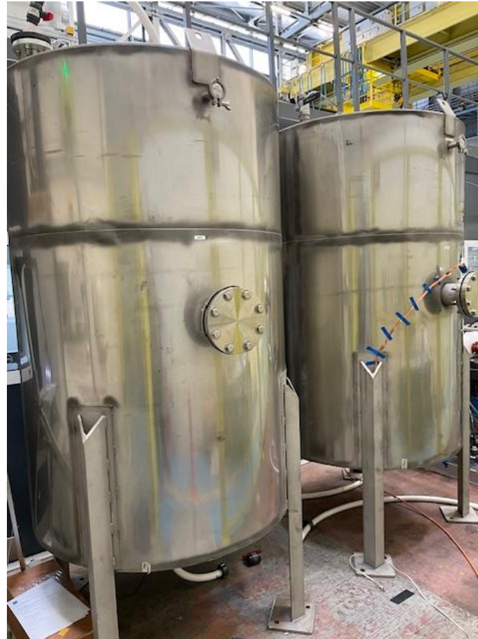
Tanks for the mixing in and extraction of Gadolinium provided by Uppsala University
