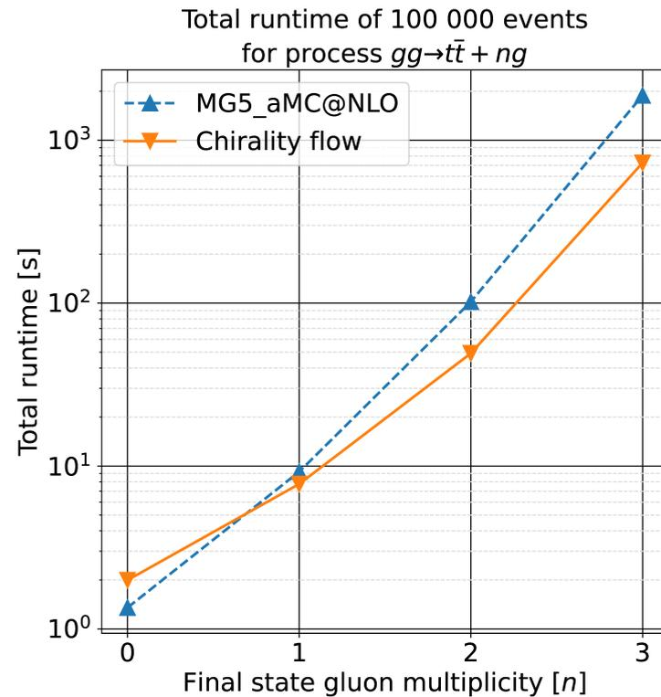
Runtime for the Lorentz structure of  $gg \rightarrow t\bar{t} + ng$ , for the standalone version of MadGraph5\_aMC@NLO and for the chirality-flow branch. (E. Boman, A. Lifson, M. Sjodahl, A. Warnerbring, Z. Wettersten, 2312.07447 (JHEP))
