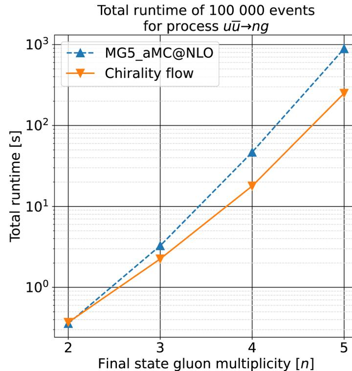
Runtime for the Lorentz structure of  $u\bar{u} \rightarrow ng$  for the standalone version of MadGraph5\_aMC@NLO and for the chirality-flow branch.
