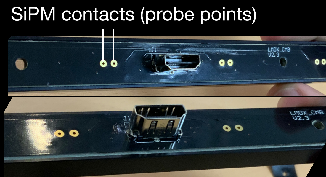
Backside of control board, showing HDMI port & SiPM probe points
