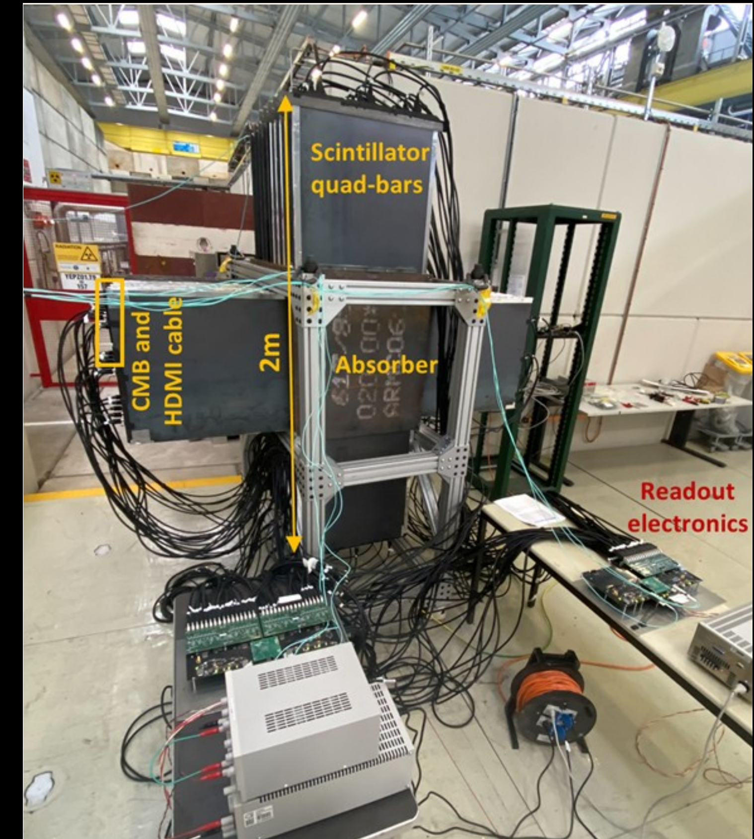
HCal prototype from CERN testbeam; now at SLAC
