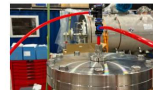
Data recorder · instrumentation panel · pressure transmitter and sensor · thermocouple and air inlet on the top flange.
