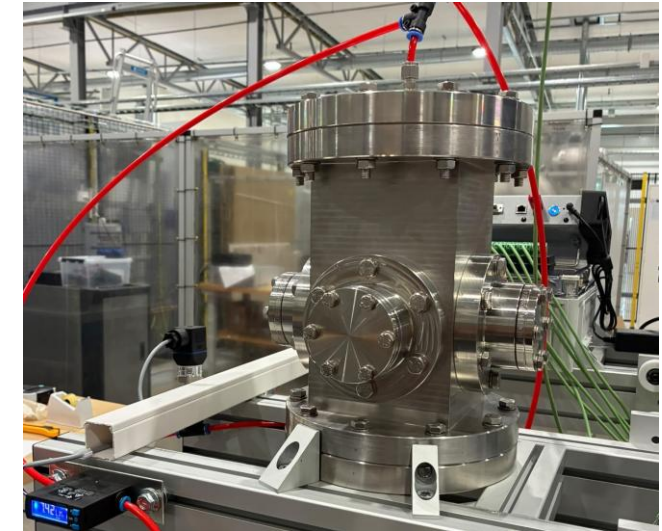
ETTF vessel on the air-test stand (ESS MML); the stand ready for the campaign.
