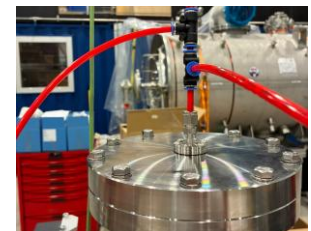
Data recorder · instrumentation panel · pressure transmitter and sensor · thermocouple and air inlet on the top flange.
