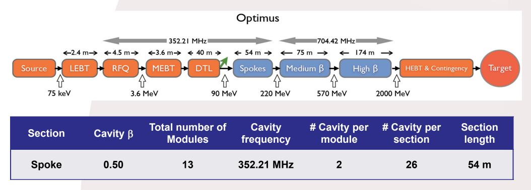
Main consequences for the spoke coming from the cost reduction effort (-> Optimus design) is the increased gradient and increased power to be transmitted to the beam
