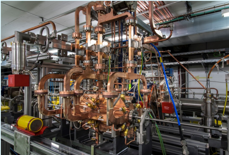
Two Beam Test Stand at CTF3 100 MV/m first demonstrated
