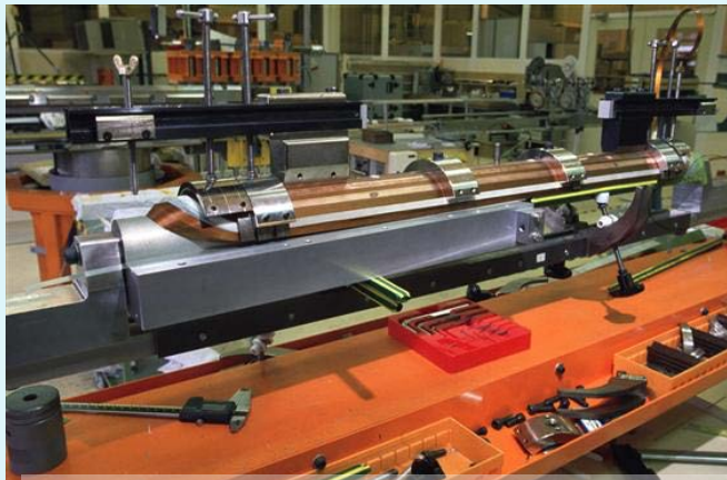
Orbit corrector magnet coil winding 20 magnets to be tested
