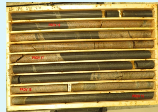
Granite drill cores
