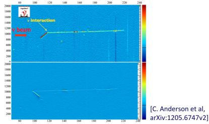
A time projection chamber with charge and light readout
