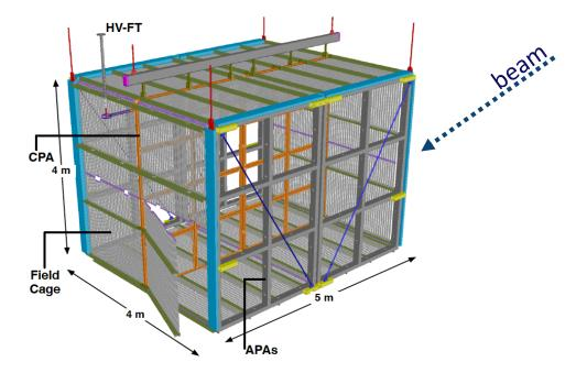
□ TPC with central cathode and 2 drift volumes with wire plane readout
