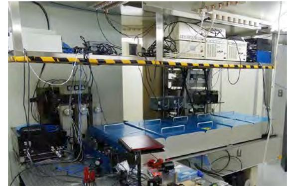
Laser was developed in collaboration with another project (USMM in U-line). Large laser crystal for main amplifier is under development in order to achieve **100  $\mu\text{J}$**  goal (10  $\mu\text{J}$  without amplifier). Will give  $\sim 75\%$  ionization efficiency in  $2 \text{ cm}^2$  laser area.
