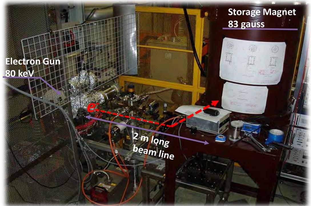
Spiral injection test with mini-solenoid and electron gun - in progress (observed two turns)
