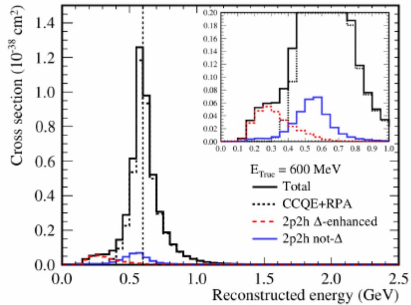
FIG. 5. Neutrino energy calculated with the CCQE two-body assumption for CCQE and 2p2h interactions of 600 MeV muon neutrinos on  $^{12}\text{C}$  simulated with the reference model. The different components of 2p2h show differing amounts of bias.
