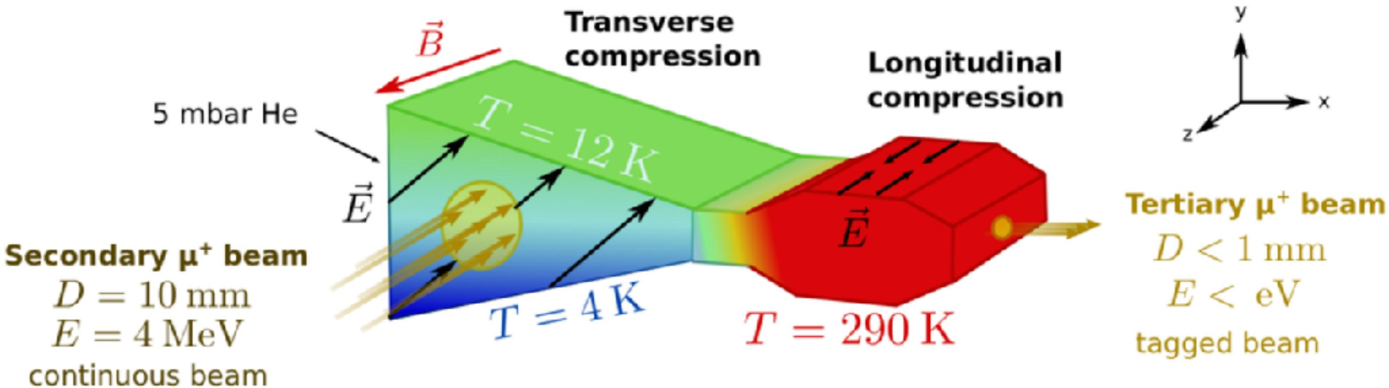
Muon swarm compression inside a He gas target employing position-dependent muon drift velocity.
