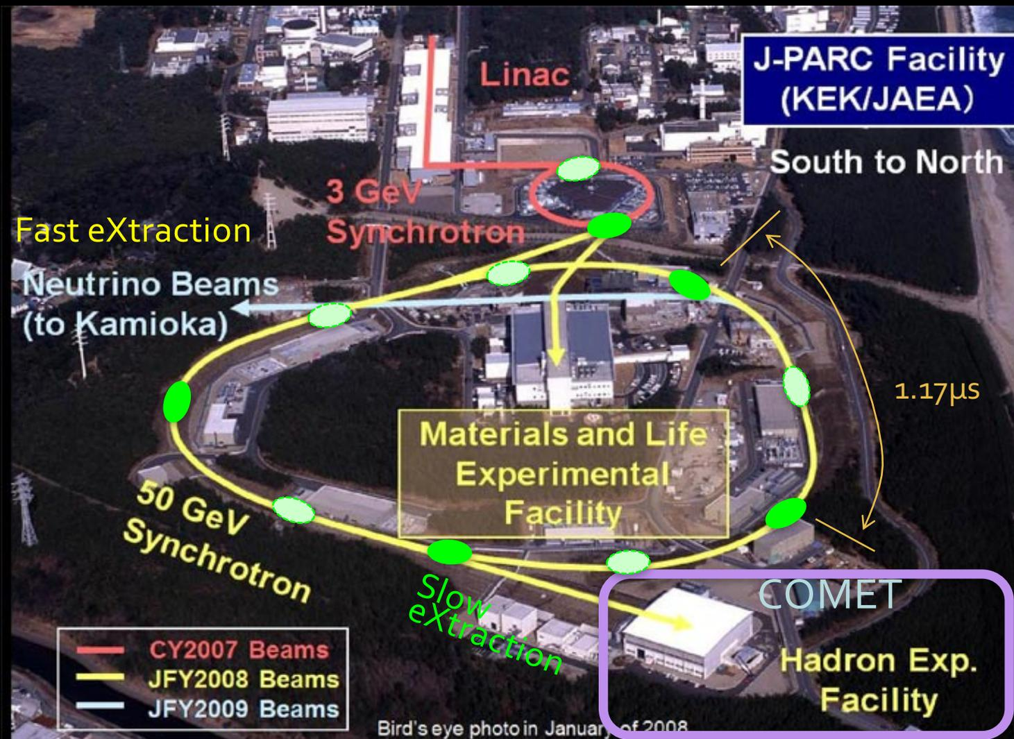
8GeV, 3.2kW pulsed proton beam in Phase-I, 4/9 (or 3/9) buckets filled in MR
