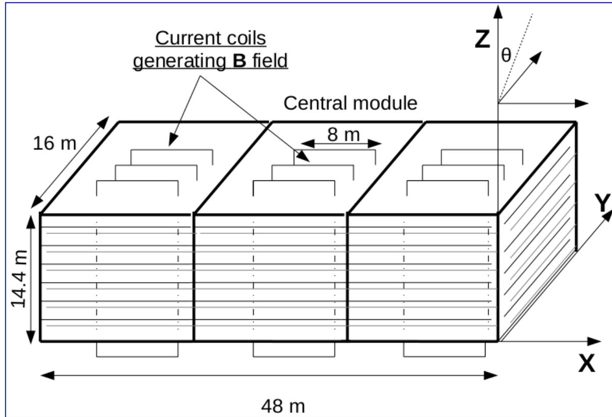
3 modules each of size  $16\text{m} \times 16\text{m} \times 14.4\text{m}$ , sampling detector with 151 layers
