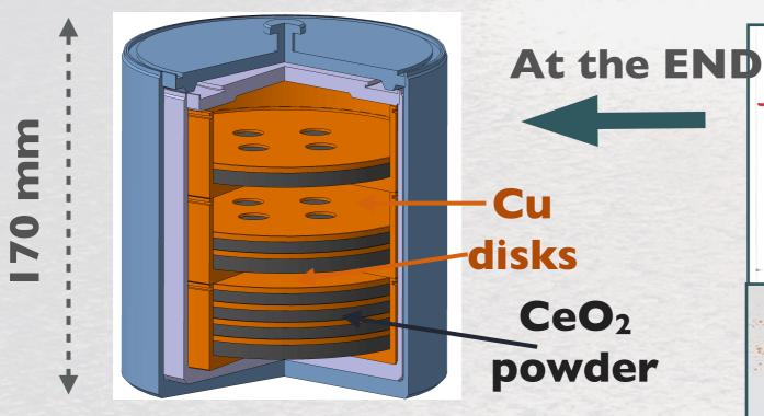
CeO<sub>2</sub> powder pressed in a sealed stainless steel capsule with copper disks for better heat transfer and internal free space for pressure control
