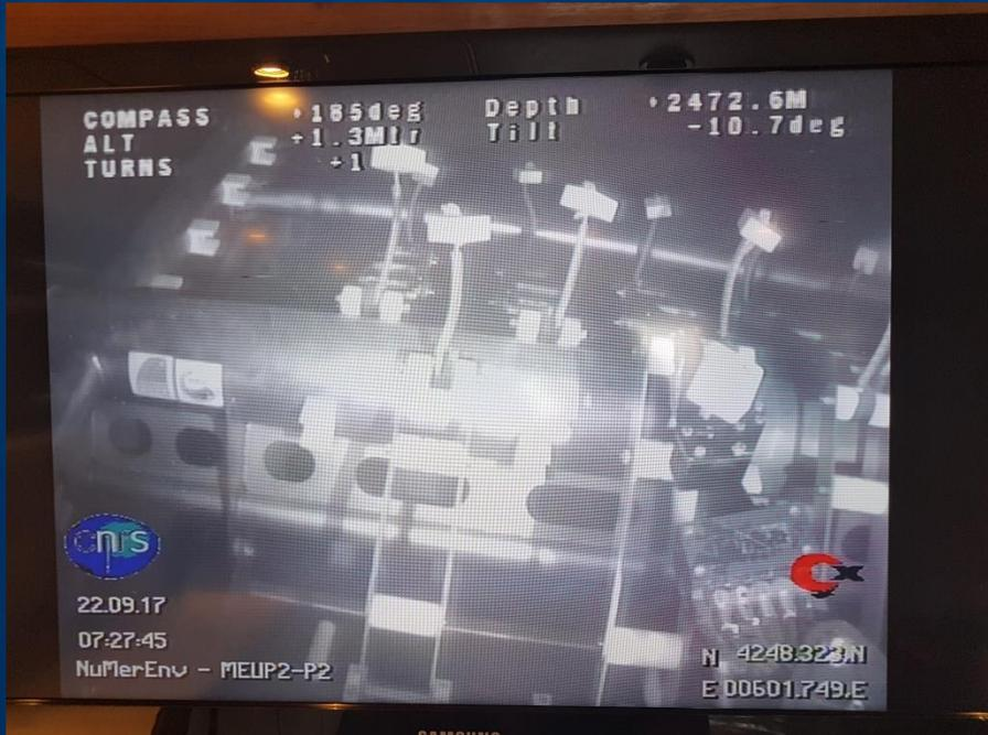
Wet-mateable connectors on the submarine node
