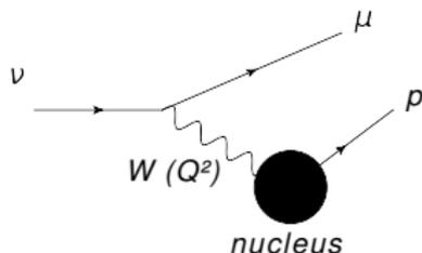
Need to measure the muon in a large phase space (in particular **high-angle** and **backward**) to estimate  $Q^2$ -dependence
