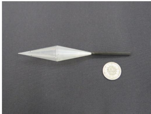
Extended hollow double-cone target
