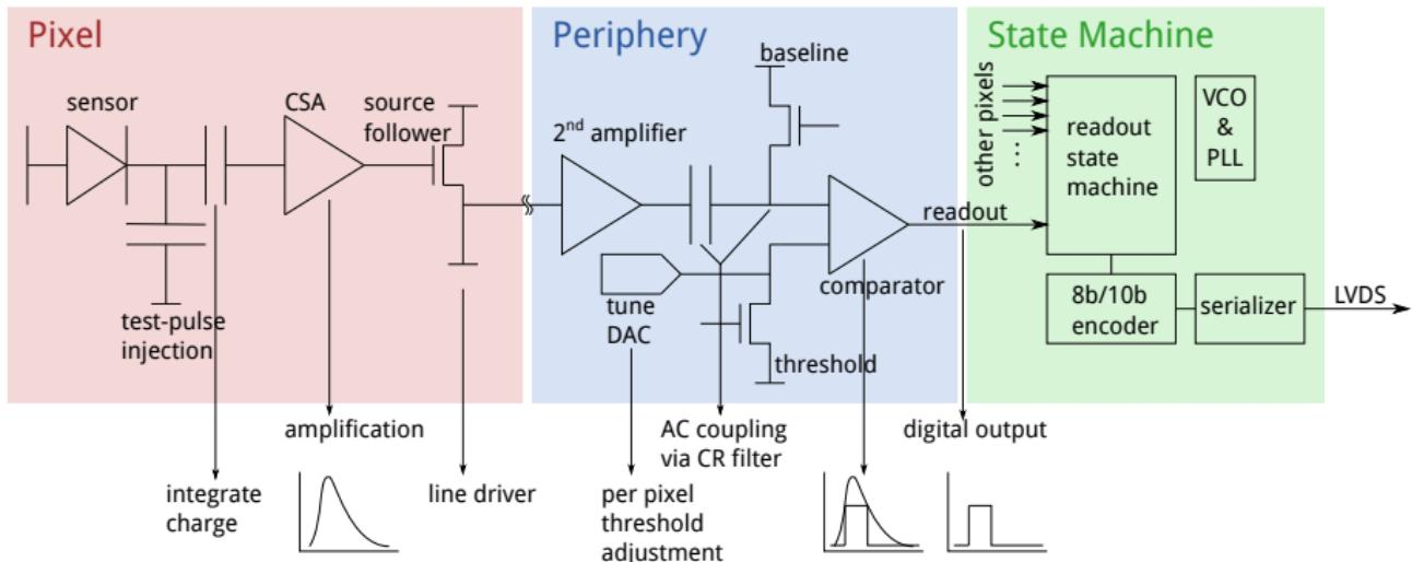
Hit finding, digitisation, zero-suppression and readout on-chip
