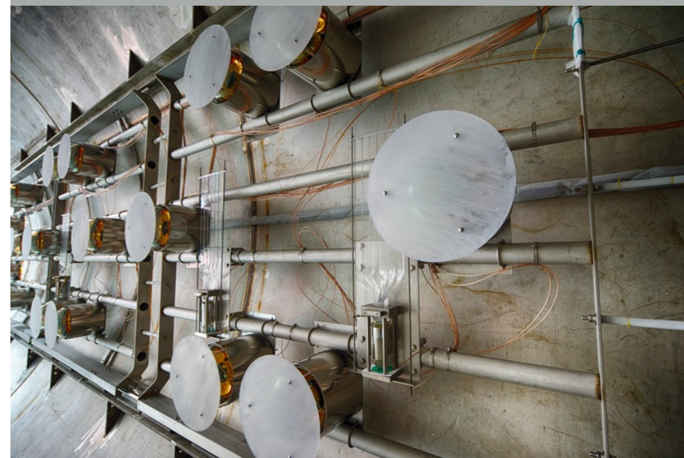
Inside the detector: PMT system
