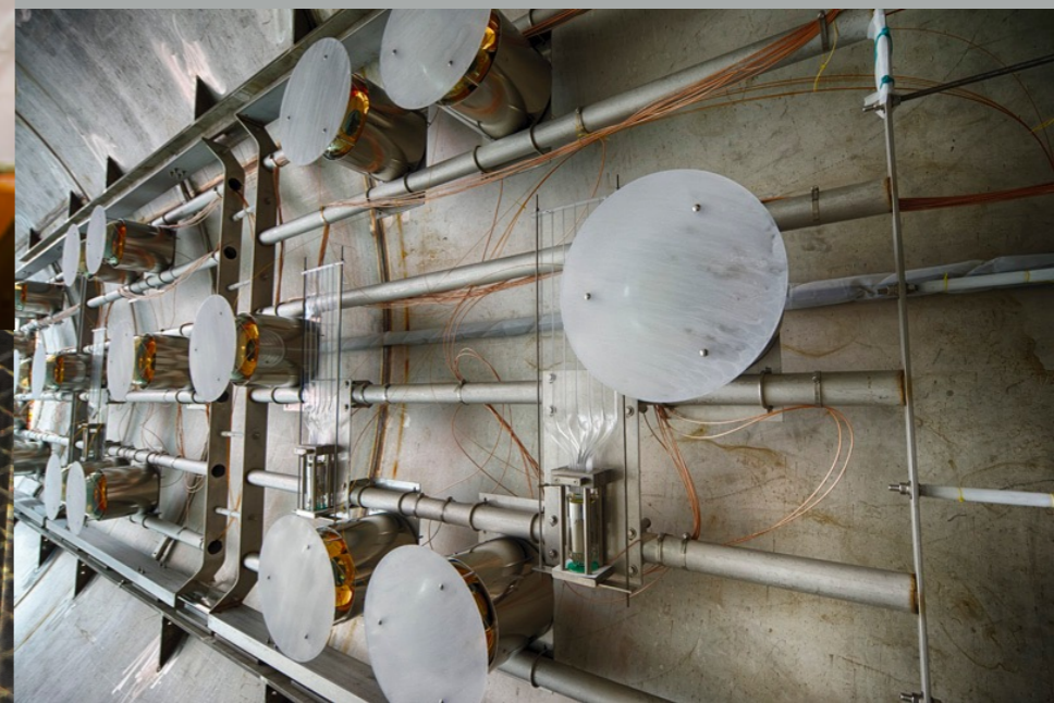
Inside the detector: PMT system
