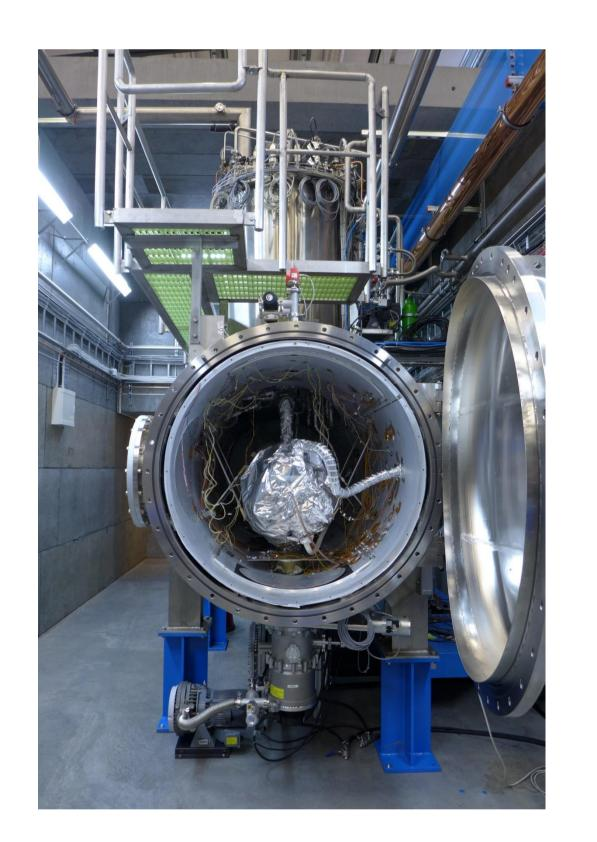
Horizontal Cryostat A versatile horizontal cryostat system for testing superconducting cavities.
