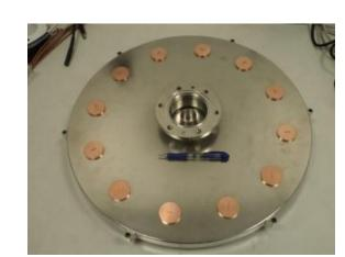
Freia Solid State Amplifier Development A high efficiency solid state amplifier, 352 MHz, 10 kW. A high efficient and compact power combiners, 10 kW and 100 kW class.
