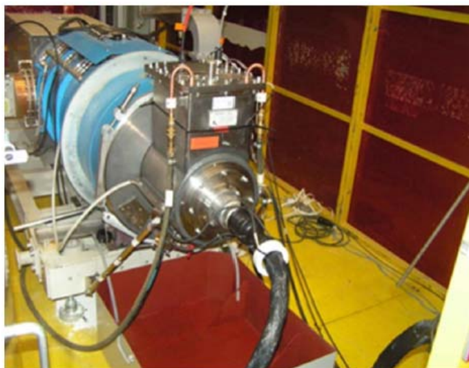
Double wall pulse transformer
