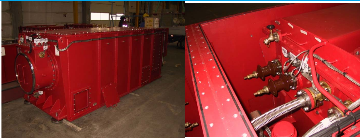
Double wall pulse transformer
