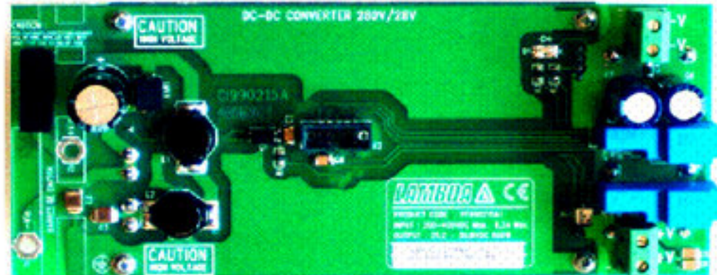
600 W – 280 Vdc / 28Vdc converter
