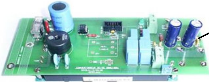
600 W, 300 Vdc / 30 Vdc converter
