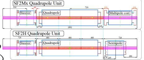
3 PCB: 5 coils  $\times$  480  $\times$  13 mm<sup>2</sup> for the main quadrupole
