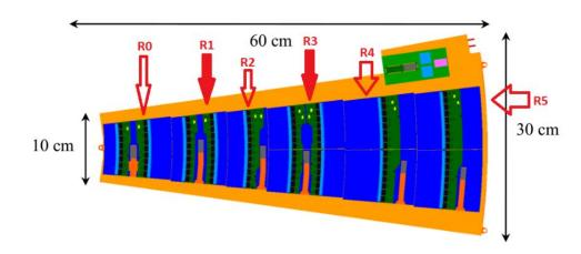
Endcap rings made of petals, based on 6 module geometries.
