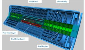
Cross section of ITK, red are pixel modules and blue strips.
