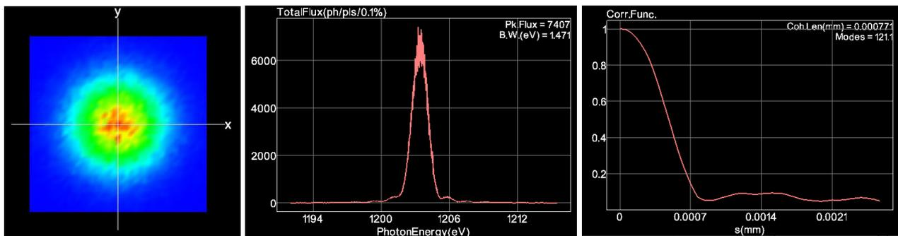
Fig. 2: Simulation results for the Compton source using the Tanaka code Simplex [5]. From left to right: the power density averaged over the pulse as a function of transverse coordinates, the photon flux per shot vs photon energy, and the temporal correlation functions of the 1<sup>st</sup> order as a function of distance.
