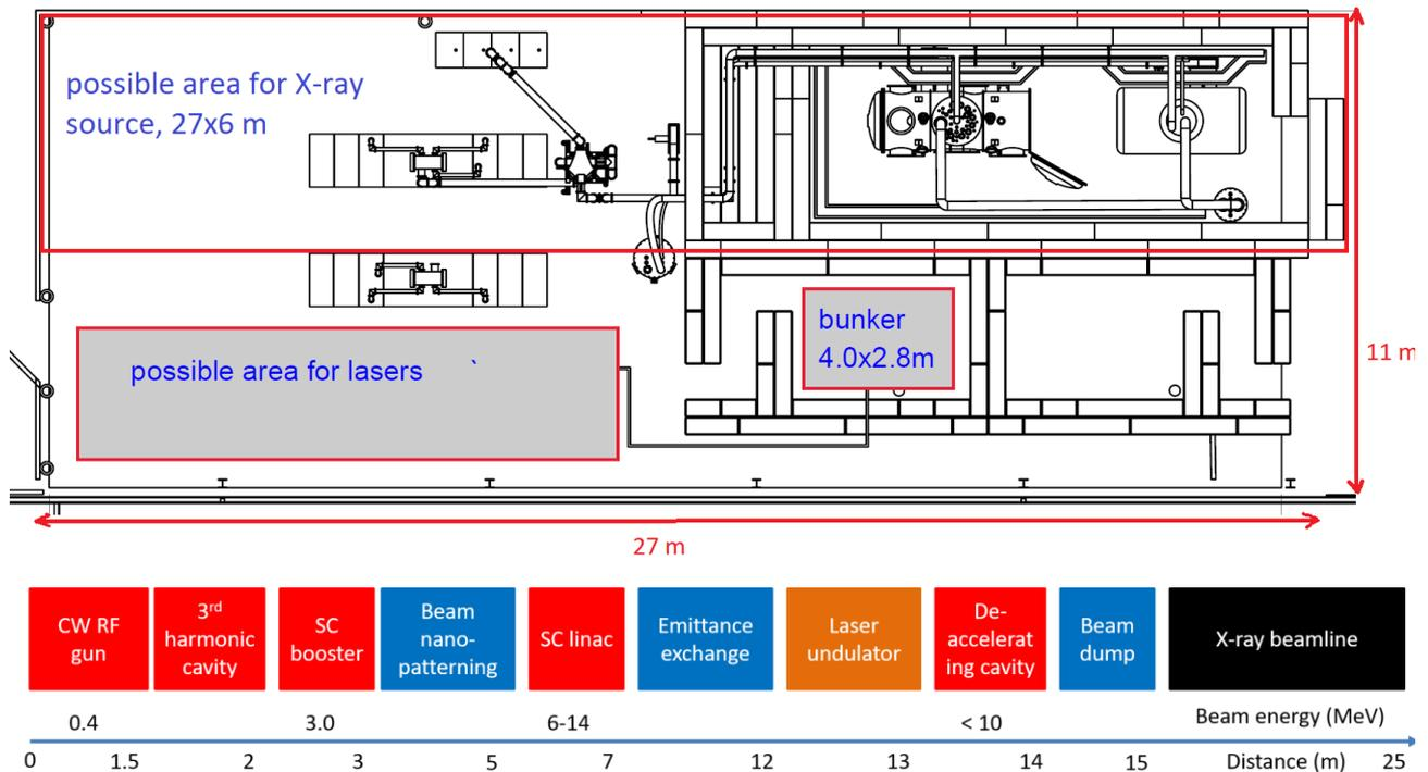
Fig. 4: Top: sketch of the total area for accelerator experiments at the FREIA laboratory. The maximum possible area for the X-ray source is 27 x 6 m. An additional area for a high-power laser along with a test bunker area are also available. Bottom: a preliminary layout of the X-ray source components.
