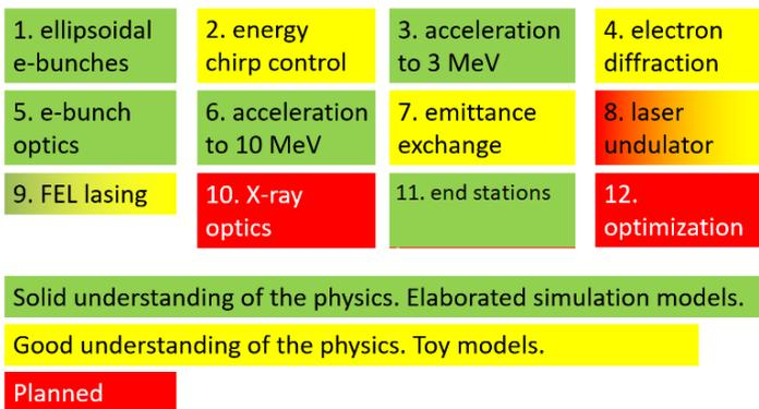
Fig. 3: High-level conceptual layout of the coherent X-ray source and a present status of S2E simulations.
