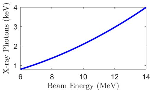
Fig. 1: Maximum energy of scattered photons vs. electron beam energy.
