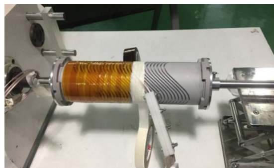
Figure 12: Winding process of the subscale quadrupole coil.
