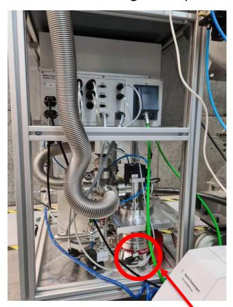
Leak detector background 2E-7 mbar.l/s Leak signal 2.4E-6 mbar.l/s
