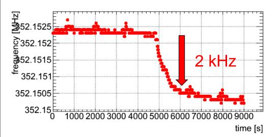
We tried to move the stepper motor backward after disengagement
