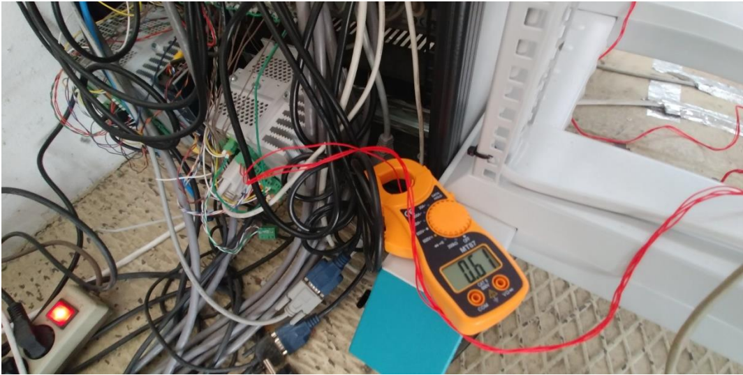
0.61 A Measured on Phytron driver output
